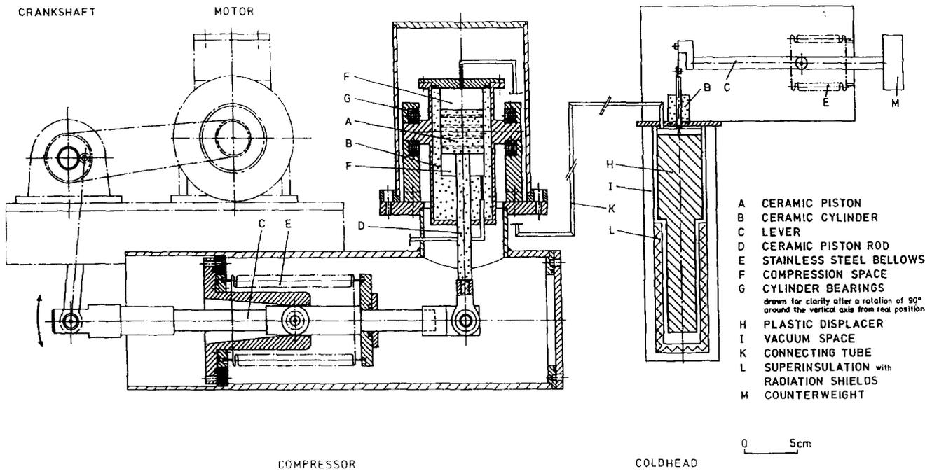
Figure 2 Two-stage split Stirling cryocooler
