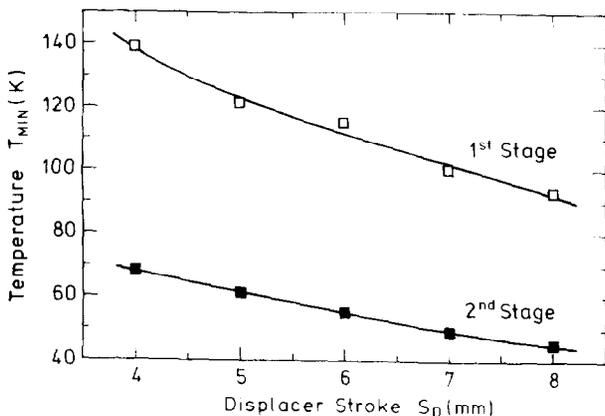
**Figure 6** Effect of displacer stroke on minimum temperature
