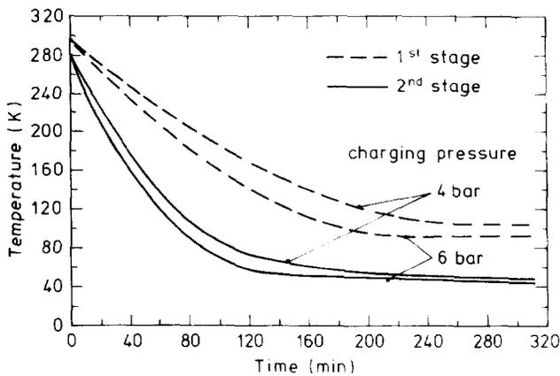
Figure 3 Cooling curves for two-stage Stirling cryocooler
