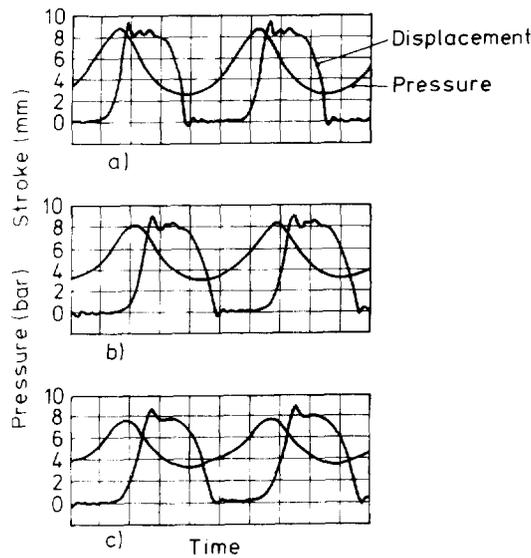
Figure 4 Pressure-displacement diagram for different 2nd stage temperatures: (a) 250 K, (b) 100 K, (c) 50 K
