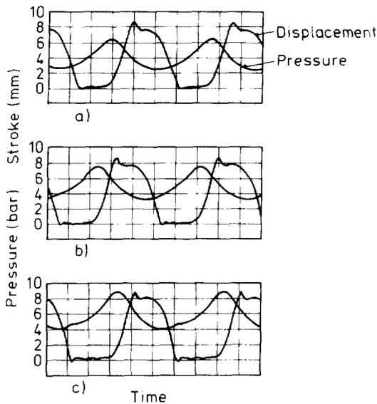
Figure 5 Pressure-displacement diagrams for different charging pressures: (a) 4 bar, (b) 5 bar, (c) 6 bar
