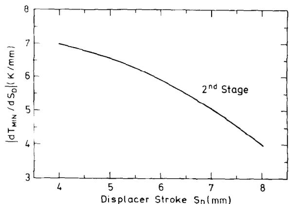
**Figure 7** Variation of  $(dT_{MIN}/dS_D)$  with stroke
